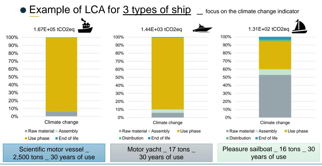
Over the lifecycle of a ship, the installation of an engine makes the use phase the main source of impact on climate change, and therefore an eco-design lever to work on.
